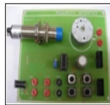
Proximity Sensor Interface
